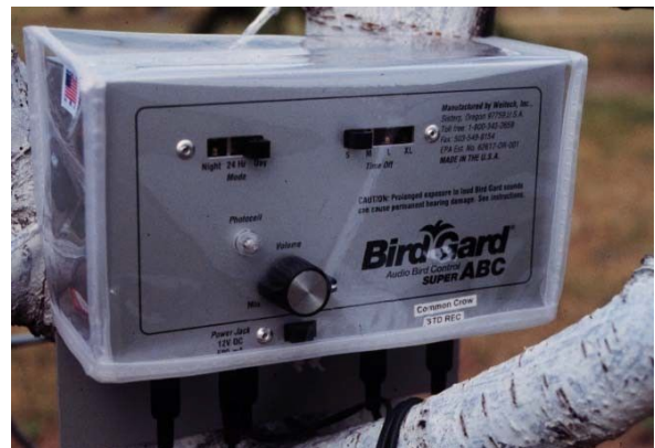
Figure 6. Device using both bird distress calls and raptor calls to deter birds from fruit crops. Image by Paul D. Curtis.
