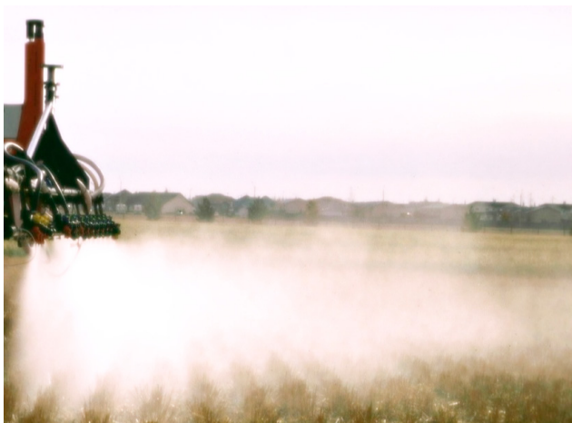
Figure 2. Standard hydraulic flat-fan nozzles at 40 psi. Photo credit: Wolf, 1999.
