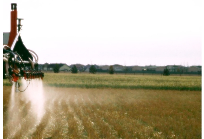
Figure 3. Air induction nozzles at 70 psi. Photo credit: Wolf, 1999.
